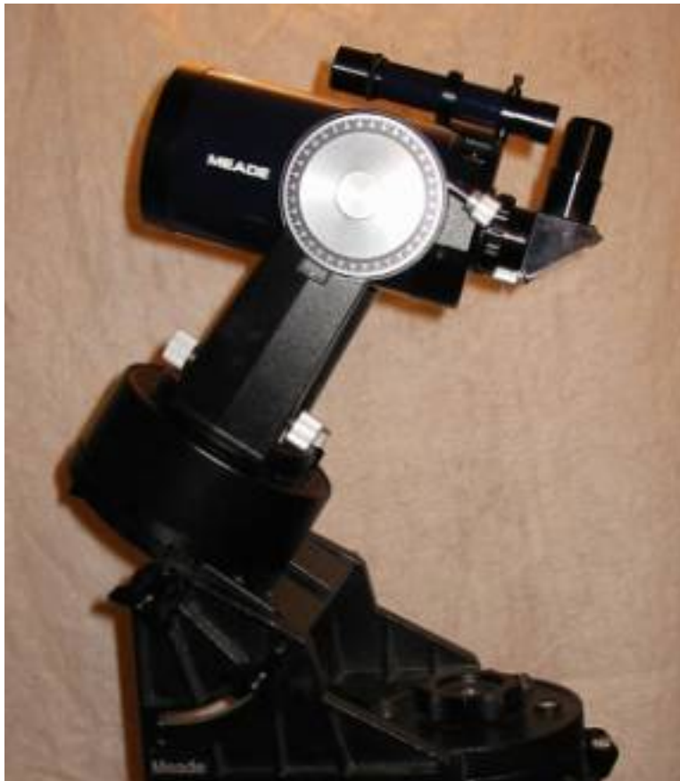
Figure 1. The Meade 2045D on its optional wedge and tripod. The scope also has three small legs so it can sit on a table top.
