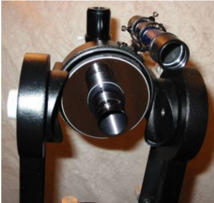
Figure 2 Here is the scope without its tube. You can see how the primary mirror slides on a central tube.
