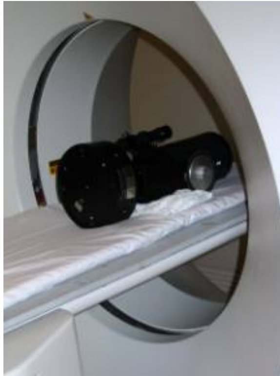
Figure 6. This is the scope in the bore of the CT scanner. The dark ring on the scanner is the location of the x-ray tube and detectors. The scan only takes a couple of minutes.
