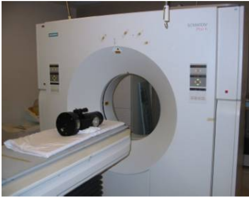
Figure 4. This is the SCT on the table of a clinical CT scanner. Note that this is not a diagnostic scanner, so no patients were denied treatment in order to scan a telescope.
